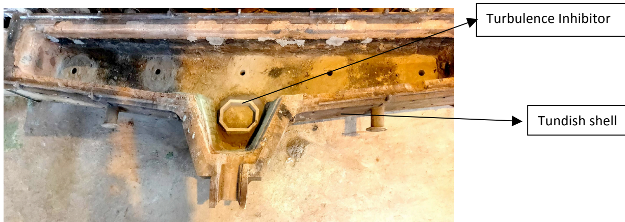
Basic structure of tundish
